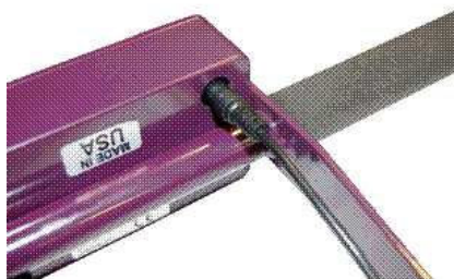
Fig. 2: Cable plugged into data port
