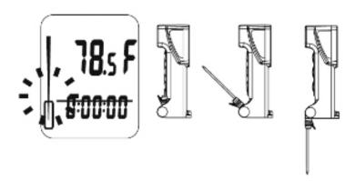
and insert into the target at least 1/2" (10mm) deep for several seconds or stir the liquid to equilibrate with the target object, and then press MEAS to measure internal temp. The probe icon blinks while measuring and stops with short beeps when the readings stabilize.
